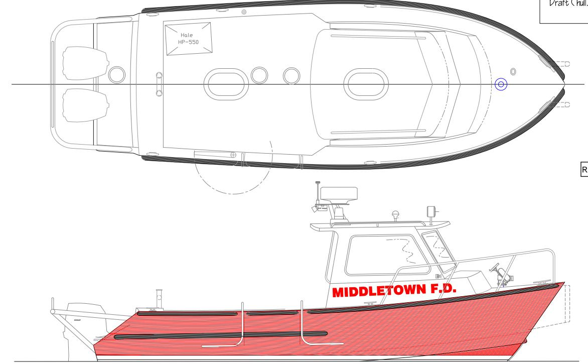
LOA(hull)- 26'0'' Beam (hull) - 9'0'' Displ. - 6,500 (Normal Operating) Draft (hull) - 1'5''
